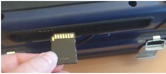
Fig. 9: Insert SD card correctly
