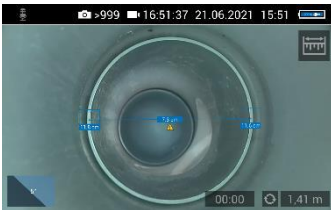
Fig. 46: Warning triangle under distance indicator
