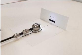
Fig. 49: Calibration with calibration template
