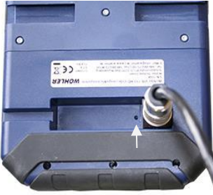
Fig. 69: Reset hole indicated by an arrow
