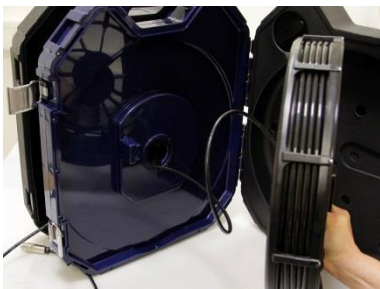
Fig. 75: Removing the viper with the connection cable from the case.
