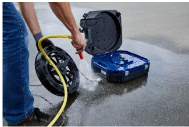
Fig. 77: Cleaning the viper and the rod
