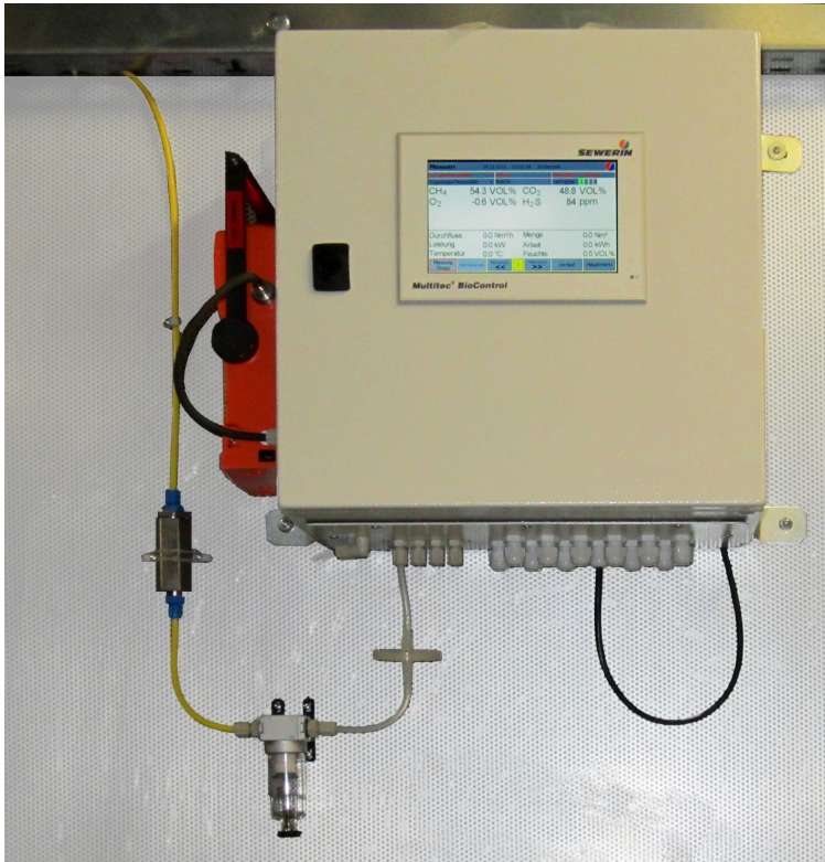
Fig. 4: Sample installation – BioControl 4 with one measurement location connected
