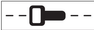
Fig. 14: Receiver oriented to the assumed route of the line for passive location
