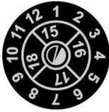
The inspection plate on the device shows confirmation of the last maintenance and the next scheduled maintenance.
